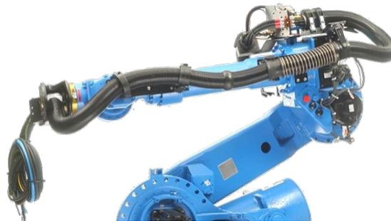
Solution 2: Energy conduit system with spring guide
