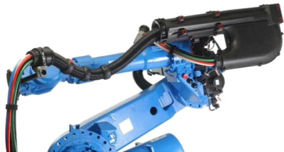
Solution 1: Energy conduit system with R-TecBox
