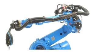
Solution 2: Energy conduit system with spring guide
