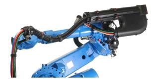
Solution 1: Energy conduit system with R-TecBox
